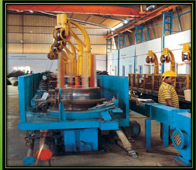
Pointing out Machine with Drum
